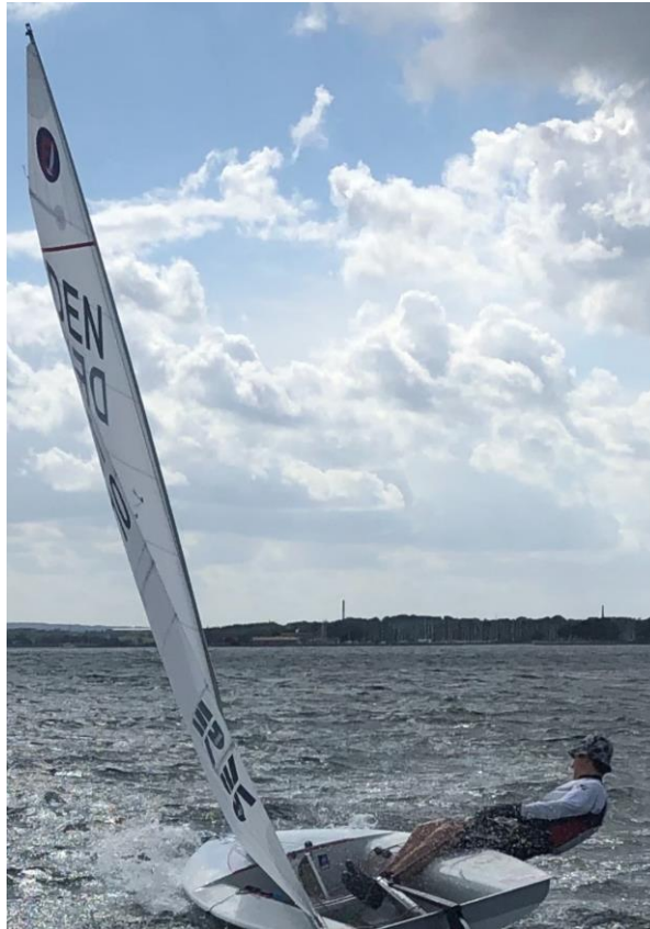
Cunningham pulled tight - the sail is twisted and open in the top
