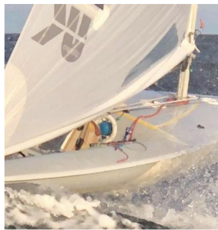
From 16 kn and over, the upper and front corner of my daggerboard is in line with the center of the inspection hatch. This is as high as my daggerboard ever comes.
