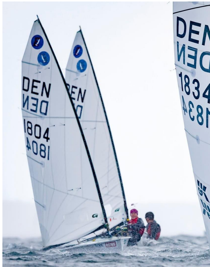
The difference between a soft and stiff mast.
